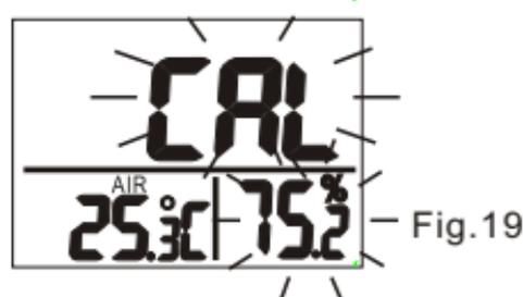
“CAL” and calibrating value (75.2% if at 25°C) are blinking on the LCD with current temperature at the left. Meter is now calibrating. Wait about 60 minutes until blinking stops, then calibration is completed and it returns to normal mode.
