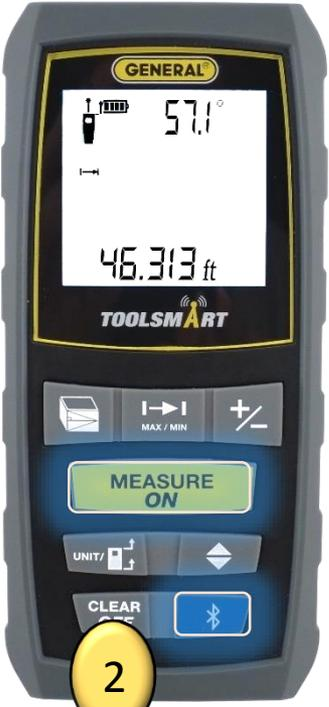
Long press Bluetooth button to turn on Bluetooth. Device will beep and "B" will start blinking on screen.
