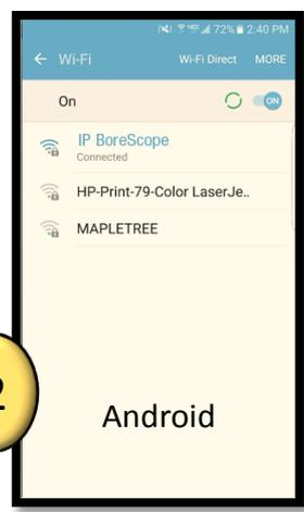
Go to Wi-Fi settings in the phone. Connect to "IP BoreScope".
